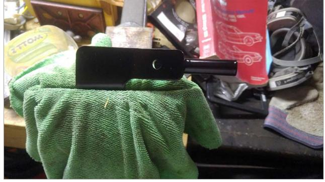
Cover the exposed face of the socket, and a couple taps with the hammer, in this case a 3# hand sledge, will give about ¼" of additional bend to the piece.
